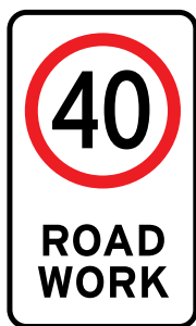
40 km/h speed limit for road works.
